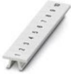
Zack marker strip, Strip, white, labeled, printed horizontally: consecutive numbers 1 ... 10, 11 ... 20, etc. up to 491 ... 500, mounting type: snap into tall marker groove, for terminal block width: 5.2 mm, lettering field size: 5.15 x 10.5 mm, Number of individual labels: 10
