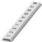
Zack Marker strip, flat, Strip, white, labeled, printed horizontally: Odd numbers 1 - 19, 21 - 39, etc. up to 81 - 99, mounting type: snap into flat marker groove, for terminal block width: 5 mm, lettering field size: 5.15 x 5.15 mm, Number of individual labels: 10
