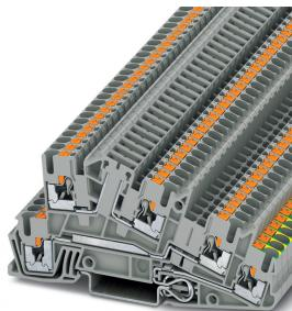
Installation ground terminal block, nom. voltage: 400 V, nominal current: 24 A, Push-in connection, Rated cross section: 4 mm<sup>2</sup>, cross section: 0.14 mm<sup>2</sup> - 4 mm<sup>2</sup>, Push-in connection, Rated cross section: 1.5 mm<sup>2</sup>, cross section: 0.14 mm<sup>2</sup> - 4 mm<sup>2</sup>, mounting type: NS 35/7,5, NS 35/15, color: gray
